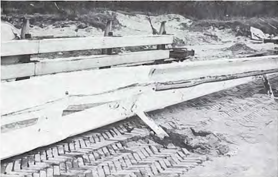
Figure 8. Impact with posts with a badly bent single offset rail barrier.
