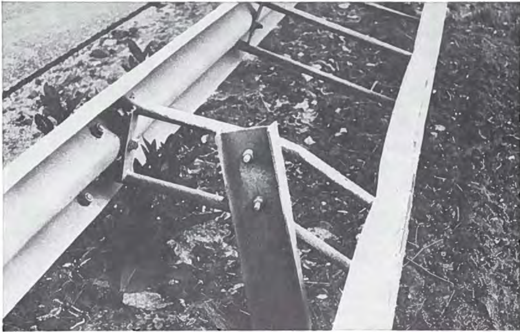
Figure 20. Front rail pressed down with insufficiently stiff spacer.
