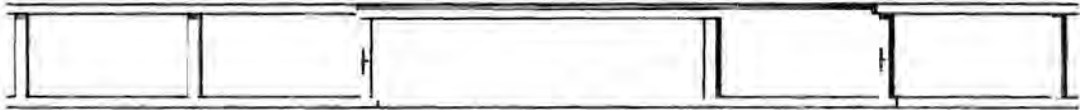
Figure 9. Model when a narrow obstacle is inside the deflection area behind a two offset rail barrier.
