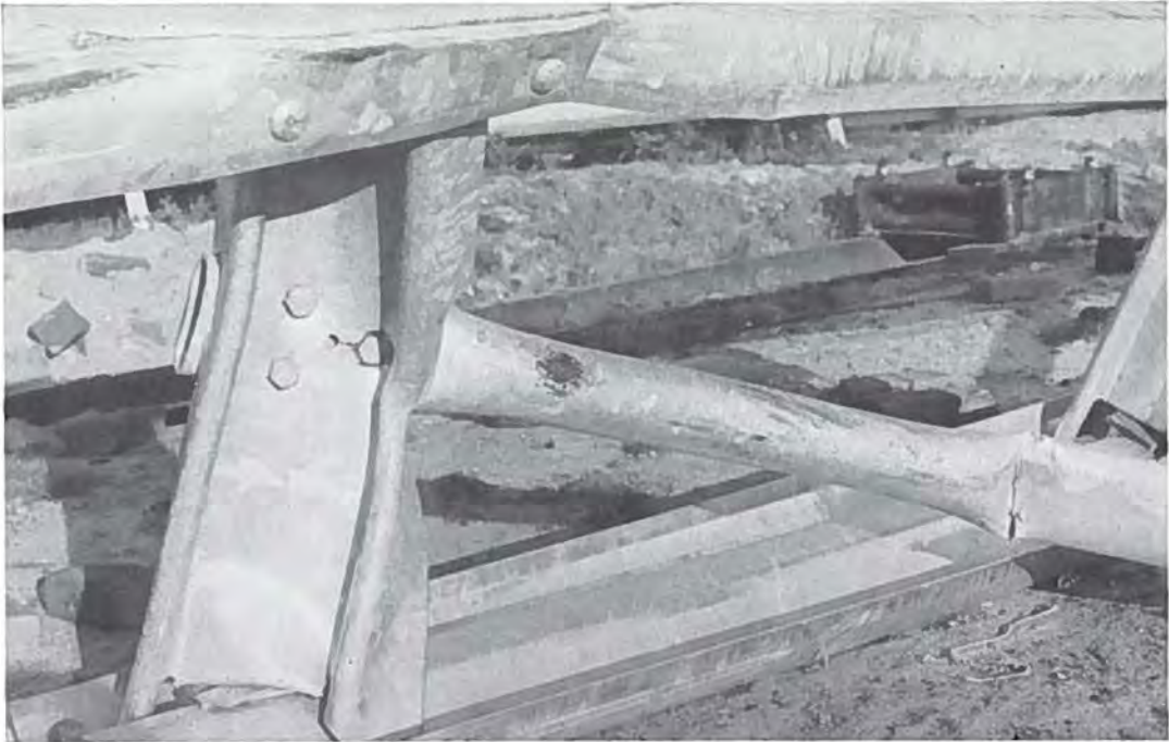
Figure 5. Impact with posts with a badly twisted beam .
