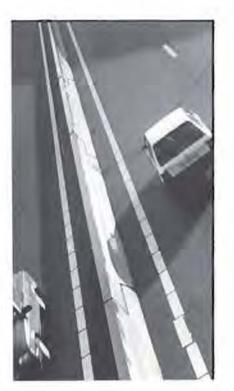
type of barrier seems to function adequately, it is neverthele's a sociated with a clear di advantage in that even minor collisions result in considerable damage to the vehicle. Therefore, SWOV carried out a study and also investigated a modification which is intended to allow the impact of minor collisions to be transferred via the wheels avoiding marked contact between the barrier and the body of the vehicle.
