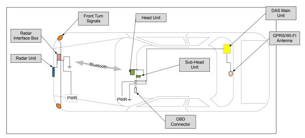
Figure 1. Parts of the Data Acquisition System (DAS) of the Naturalistic Driving study in the United States (Dingus, 2008).
