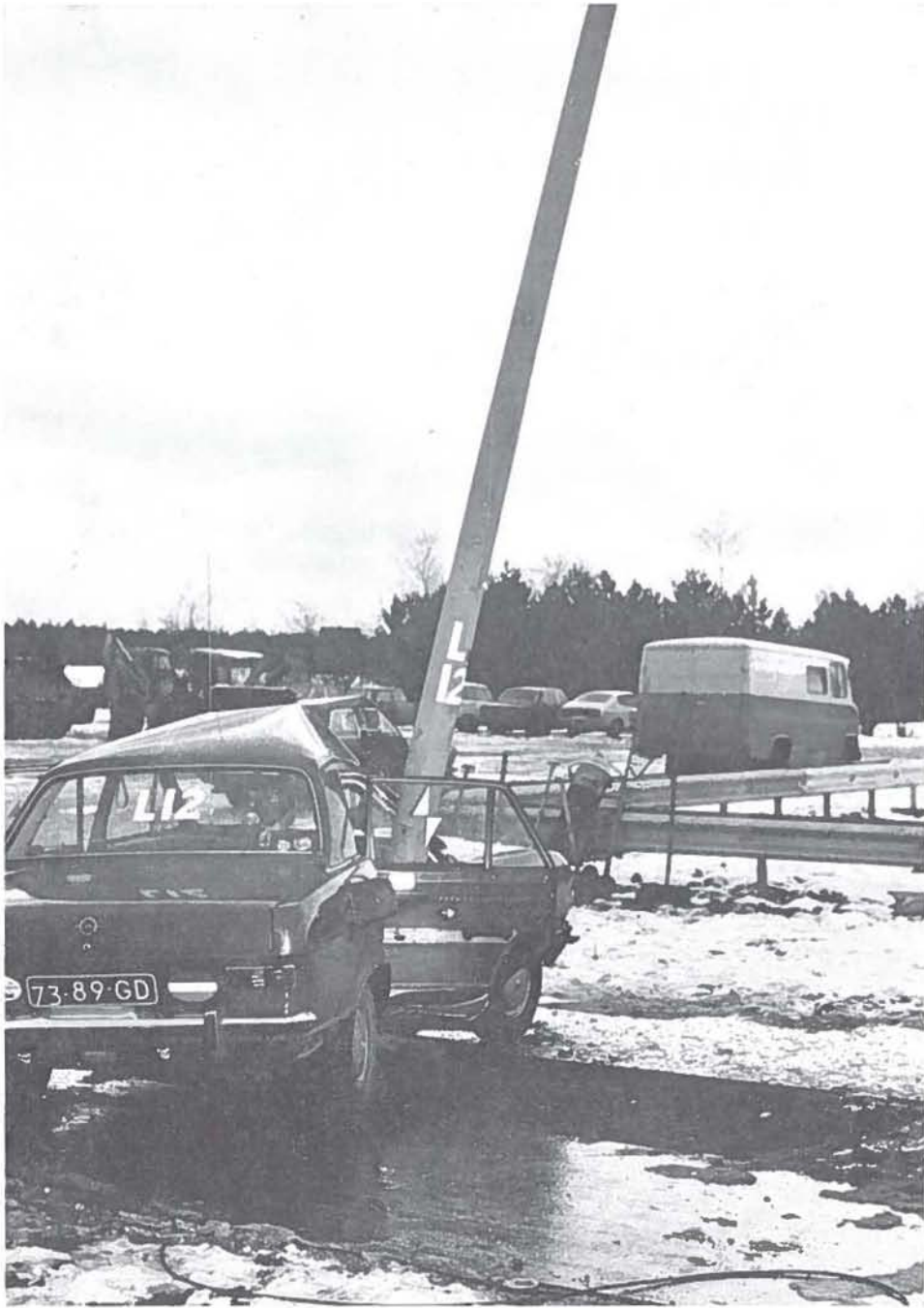
In order to examine the danger of sideways-on collisions during the research into Lighting columns, a special test installation was used with which reproducible lateral impact tests can be made.
