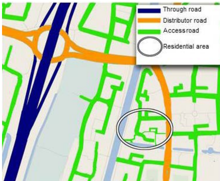
Figure 1. Three functional road types as the basis of a sustainably safe road traffic
