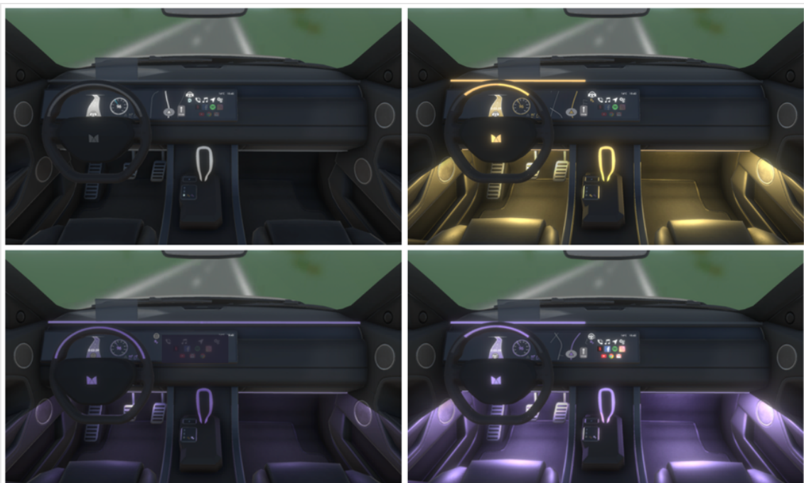
Figure 2.2 Mode awareness through ambience, clockwise from top-left: manual, assisted, piloted and piloted dark mode.
